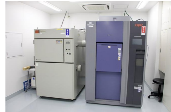
Thermal cycling chamber
